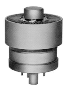
The 4C350FJ/8904 is intended for Class AB linear RF amplifier service. The tube has rugged internal construction features. The 4CX350FJ/8904 may be used as an exact replacement for the 4CX350F/8322 in most linear applications, requiring only minor circuit adjustment and retuning. The tube has improved intermodulation distortion characteristics. It contains a 26.5 volt heater and is recommended for new equipment designs.
